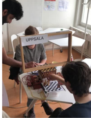
Figure 15: Prototype 6 - "Wizard of Oz" approach to mimic automated chess board
